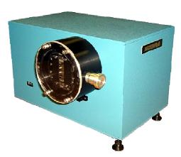
Efficiency is good with a high throughput prism material and the 303's toroidal optics. Dispersion varies with the index of refraction of the
