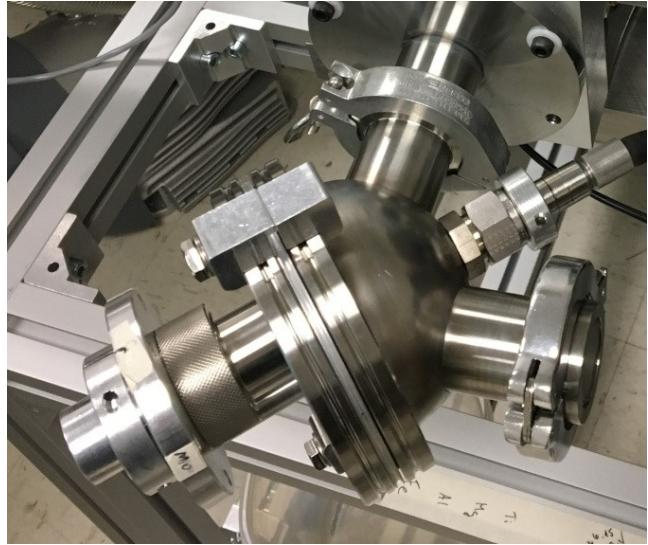
The new controller is an easy to use high voltage power supply and e-beam emitting filament current controller. It provides integrated and safety interlocked control of the electron impact soft x-ray light source. A dedicated cable connects the controller to the light source's vacuum enclosure.
