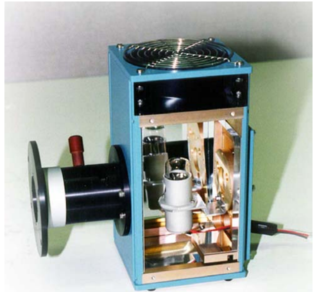
Model 621 Lamp Housing with Deuterium Lamp Installed (Model 732-1 power supply not shown)
