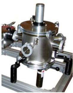
The sample chamber allows (goniometric) independent positioning of the sample and detector. Set the angle even while
