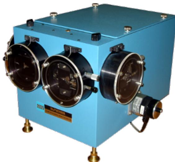
Use the 2035 monochromator for research or teaching. It is great for applications like Raman, luminescence, fluorescence, reflection and transmission.
