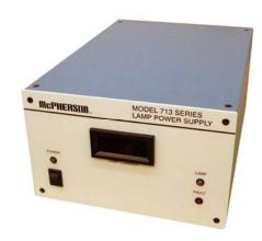
"At-a-glance" indicators on the front of the unit show lamp status and current being drawn by the lamp. Shielded external Igniter Box with all cabling supplied. Safety interlock system disables the power supply if the fan cable is not connected or if an interlock switch on the lamp enclosure (McPherson or customer-provided) is activated. Unit produces 24VDC to drive external cooling fans.
