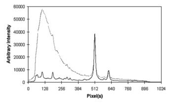
On grazing incidence spectrometers sometimes "noise" caused by stray electrons and ions overwhelms the signal of interest. Use of a suppression voltage eliminates this unwanted contribution. The graph above left shows electron noise as a gray line eliminated from the spectra (black) by applying a low negative voltage to the face of the microchannel plate. The suppression feature is standard in the Model 735 microchannel plate power supply.
