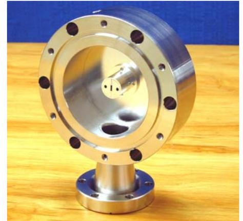
With a 0.12 x 2 inch long aperture conductance is 0.063 liters per second for air. This provides a pressure differential of ~1,500 if the high vacuum side is pumped with a 100 liter per second pump. The pressure ratio increases linearly with the speed of the high vacuum pump.
