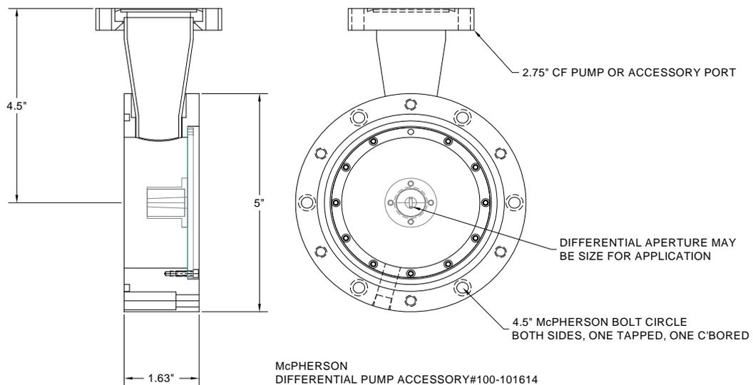
A general rule of thumb for estimating conductance of air considers the length (L) and cross section (D) of the limiting aperture. Then,  $\text{conductance} = (73 * D^3) / L$ . This approximation is valid for conductance of air and when the units for D and L are inches.
