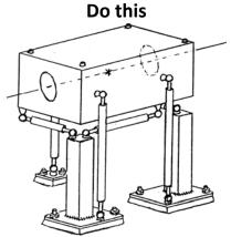
The struts are long and well separated. Two simple pedestals are tucked under the equipment to maintain a narrow footprint. The lower and upper faces of the equipment are kept clear
